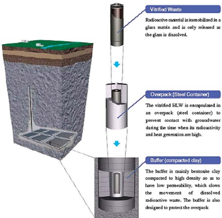
Figure 16.13 Schematic diagram of the final steps in putting vitrified waste into a geologic repository.
